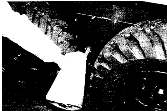
Supplying Oil to Final Reduction Gear
