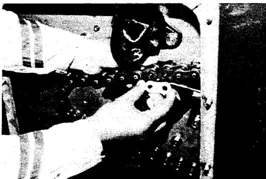
Disconnecting the Rear Drive Chain
