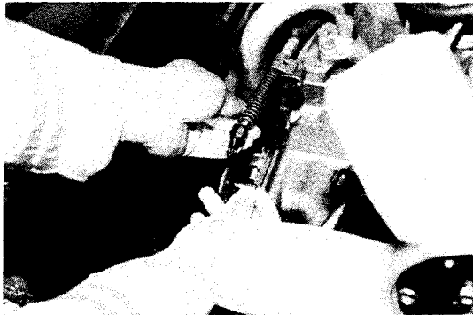
Disconnecting the Accelerator Wire
