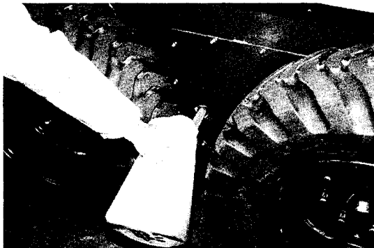
Supplying Oil to Final Reduction Gear
